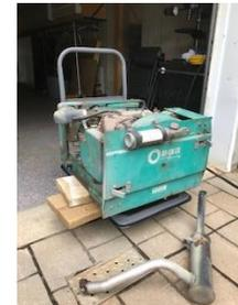
*The next removal was the Onan drawer unit itself. This is attached right to the main frame of the coach with four large bolts and hex nuts. Penetrating oil along with a heavy duty air-powered impact wrench solved the 40+ year old rusted bolts without too much trouble.*
